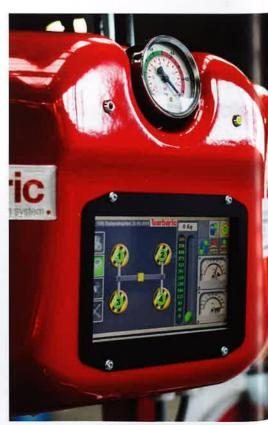
With these modern control units, vacuum lifters can also prompt the user to perform a mandatory safety check during daily start-up of the system. Step by step, the control unit guides the user through the visual inspection as well as a function check, making sure all vital functions of the lifter are operating at the highest possible safety standard.
